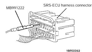
SRS-ECU harness connector (rear side)
